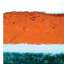
(Cross-section of cadmium red on Encausticbord™ magnified)
